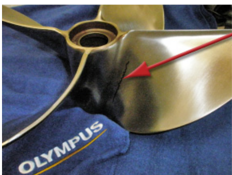
Potential location of cracks forming during high performance applications
