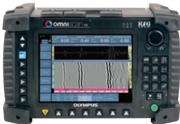
OmniScan UT with TOFD display
